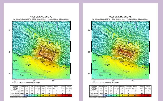
USGS "ShakeMaps" for the 2015 Gorkha (Nepal) earthquake from seismology alone (version 6; left) and incorporating geodetic observations (version 7, right). The inclusion of geodetic data results in stronger shaking over a smaller area, and increased intensity in Kathmandu.
