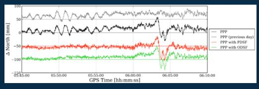
Fig. 4 - The same GPS time series for station AV24, but with the time series resulting from the two types of sidereal filter also shown. The time series on the vertical axis are offset by 50mm for clarity.
