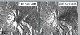
Radar backscatter images of Calbuco volcano on 14 and 26 April 2015. Differences between the two images are due to changes in the scattering and reflecting properties of the ground, caused by the deposition of explosive deposits and removal of material at the volcano's crater.
