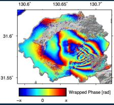
Sentinel-1 TOPS interferogram showing the deformation associated with the intrusion of a vertical planar body of magma, or dyke, in August 2015. Each colour cycle represents 2.8 cm of ground motion in the satellite line-of-sight, with the maximum deformation on the eastern side of the intrusion reaching ~14 cm
