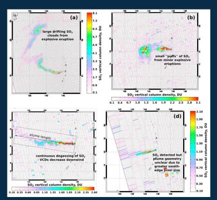
Representative daily snapshots of SO2 vertical column density over Anatahan volcano as measured by the satellite-based UV spectrometer OMI. From the geometry of SO2 clouds, we can track broad changes in style of activity. The mass of SO2 in each cloud can be computed and a timeseries of daily observations of this so-called atmospheric loading can be used as a proxy for degassing flux
