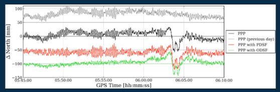
Fig. 5 - GPS time series for station AV27 including those resulting from the two types of sidereal filter. The time series on the vertical axis are offset by 50mm for clarity.
