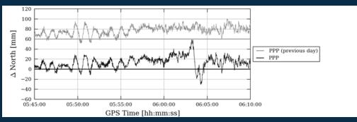
Fig. 3 - The GPS time series (North-South component) for station AV24 on the day of the earthquake and on the day before. The time series on the vertical axis are offset by 60mm for clarity.
