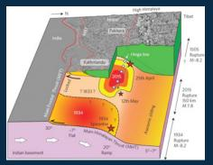
Location of the 2015 earthquake and its aftershock on the resolved Main Himalayan Thrust geometry (with the upper plate removed to reveal the slip zone). High-frequency seismic sources are marked as diamonds running along the hinge line between the ramp and flat. The Mw 7.2 aftershock occurred at the eastern end of the main rupture.
