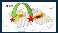
The 50 km jump imaged between the two fault planes which ruptured in the 1997 Pakistan earthquake. This leap between faults is 10 times larger than the previously though maximum.
