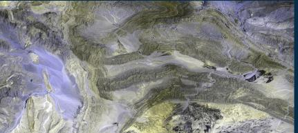
Fold and thrust belt of the western Sulaiman mountains of Pakistan. Hidden beneath these folds is the pair of large fault planes that ruptured in the 1997 Harnai earthquake, jumping 50 km between segments. Image: Landsat 8 false colour image
