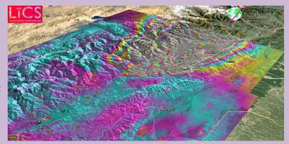
Satellite radar images of ground deformation across Nepal resulting from the 2015 Gorkha earthquake. Each coloured fringe is equivalent to 10 cm of motion, indicating the city of Kathmandu rose by over a metre whilst the highest mountains in the north sank by over 60 cm.
