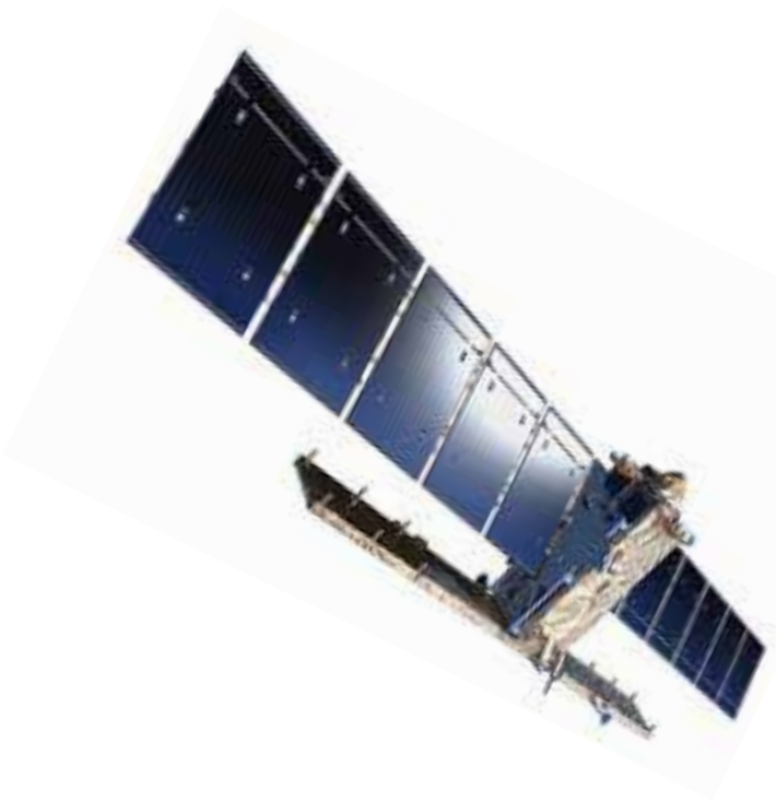
Sentinel-1A, launched in April 2014 and joined in 2016 by the identical 1B. This two satellite constellation offers the chance of 6 day revisit periods, allowing for a greater number of observations and more rapid detection of deformation
