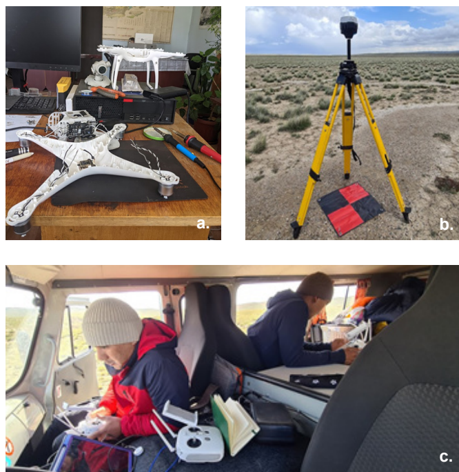
Figure 1. (a). Installing the Teokit chip and antenna into the new Phantom 4 (b) Emlid Reach RS2 setup as a base station over a GCP (c) Flying three Phantoms at once in our UAS mobile command station.
