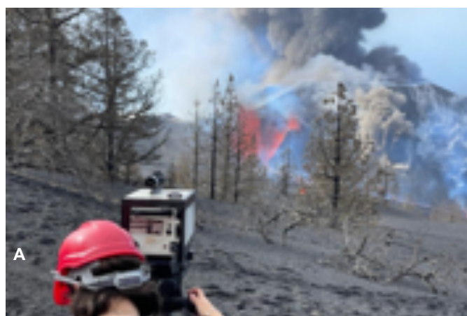
Figure 1. (a) Ana Pardo-Cofrades making FTIR measurements at Cumbre Vieja; (b) FTIR output spectra
