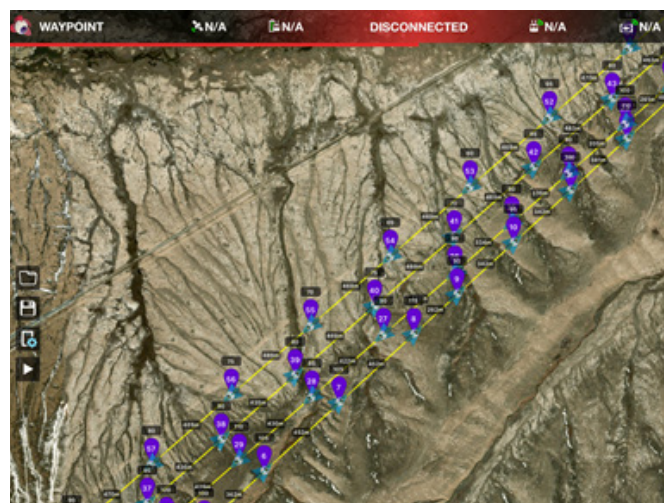
Figure 2. Screenshot from iPad showing the Litchi flight control app and a track planned using Teofly.
