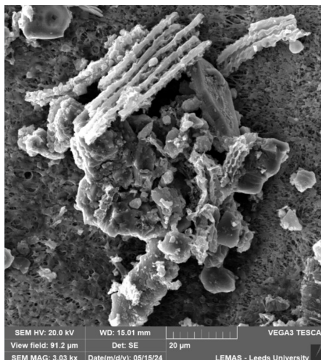
Figure 4: SEM image showing volcanically derived silicate particulate coated with fibrous burned organic matter. Sample collected in mixed volcanic-wildfire pollution along hiking path.
