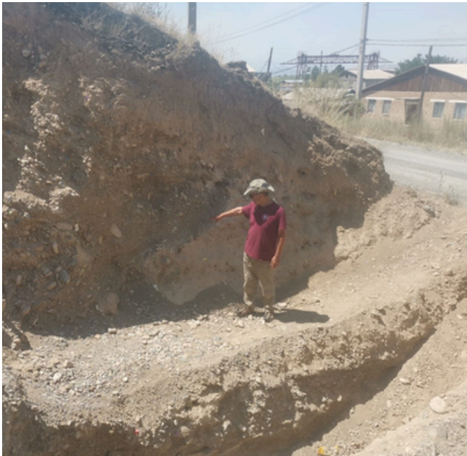
Prof. Kanatbek Abdrakhmatov (Director of the Institute of Seismology in Bishkek), pointing out a near-surface reverse fault at the trench site, Kambarata-2.
